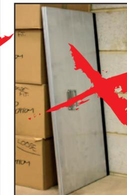
**1** Store the flood boards flat, so the board is not resting on the rubber seals either on the floor or against a side wall/surface.
