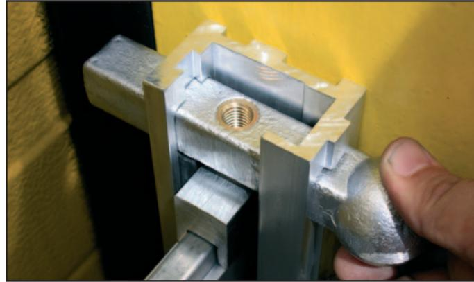
**6** On top of each compression bar, and top of the post compression casting, by hand, start turning each 12mm grub screw, clockwise, until finger tight.
