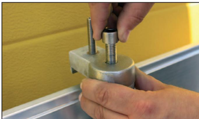
**5** Position the compression block between the top of the board and the compression retainer of the compression post, then turn the 10mm grub screw, clockwise, by hand, until finger tight.
