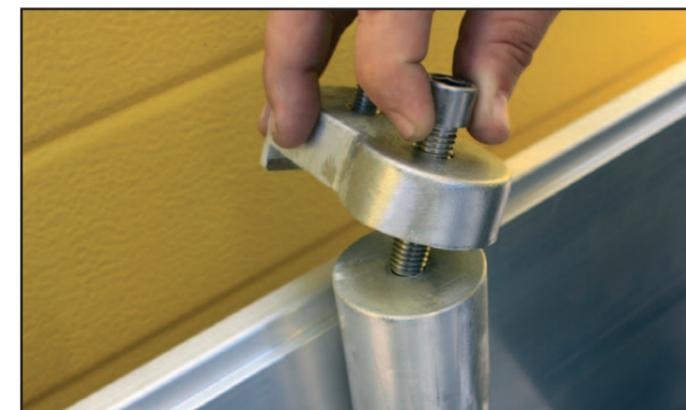
The compression post is utilised for the Nautilus® 400 barriers that spans over 1,500mm but less than 2,500mm for heights up to 1,200mm. This component ensures that adequate downward pressure is applied in the centre of the flood board and along the entire barrier span.
